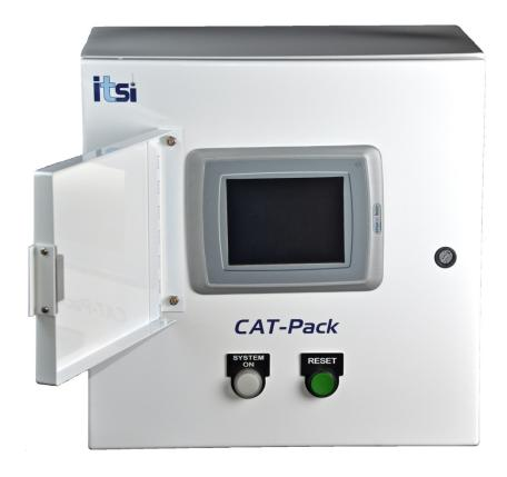
Cat-Pack provides remote monitoring of the compressor catalyst system, monitoring pre and post catalyst temperatures and differential pressure across the catalyst, O2 voltage and runtime. This data is then logged locally and provided as a local download, or can be transmitted as Modbus data to a central SCADA system.
